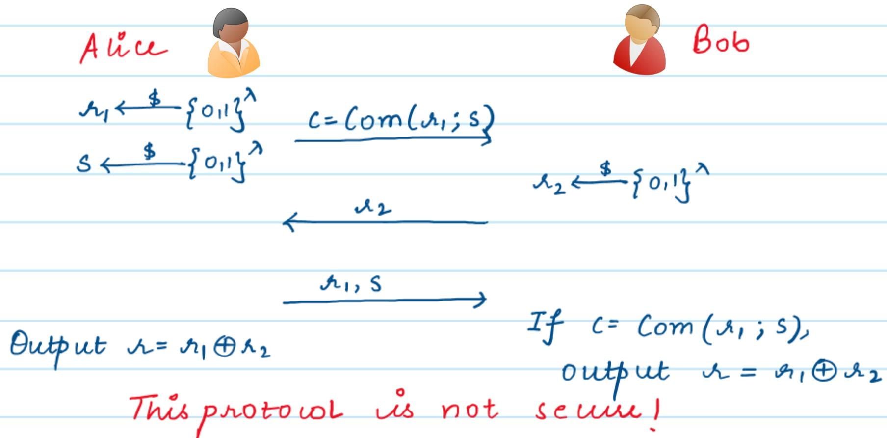
→ The simulator given a random  $r$  from fct is now unable to fix  $r_1$  such that  $r_1 \oplus r_2 = r$ , since  $r_2$  depends on  $r_1$ .
